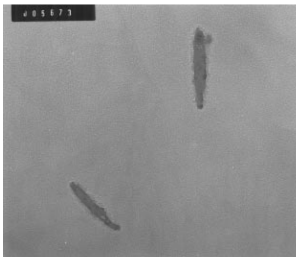
Figure 7 TEM image of magnetic SiO 2 coated \gamma -Fe 2 O 3 nanoparticles converted from the \beta -FeOOH of 24 hour hydrolysis, magnification number = 125,000.
